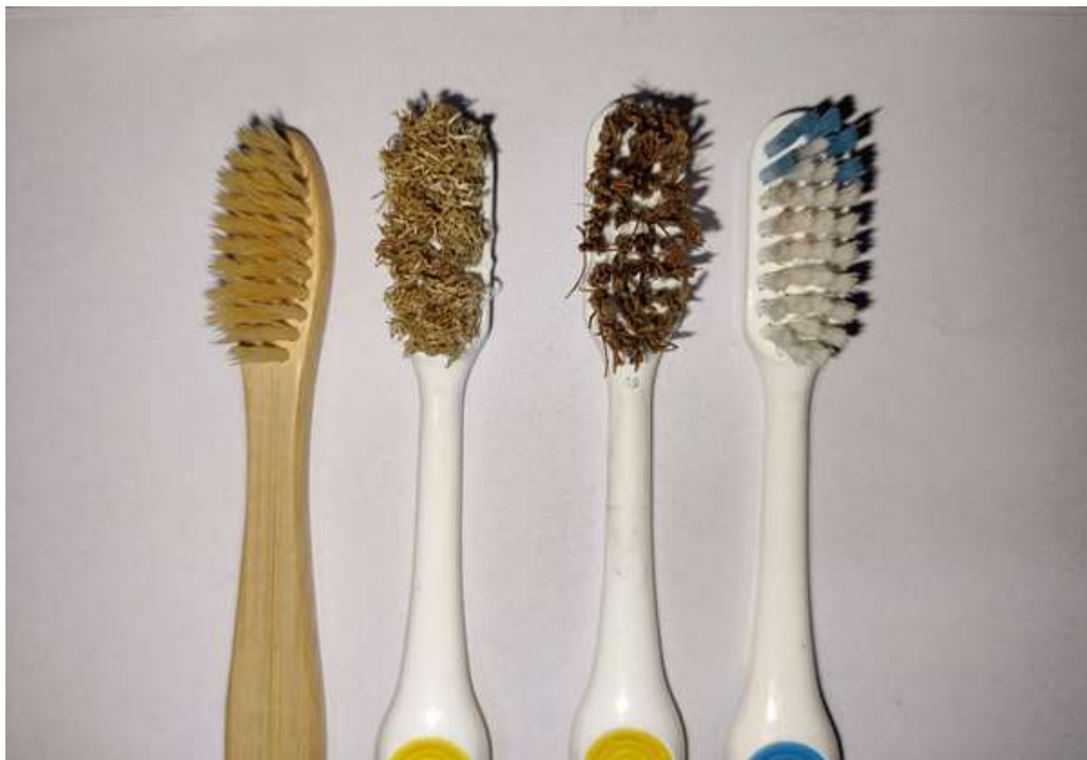
Figure 3. Different types of brushes used in order from left to right, Bamboo bristles, Ridge Gourd bristles, Coconut bristles and Nylon bristles
