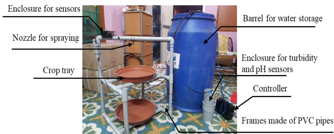
Figure 6. Prototype of entire hydroponic system with on-board display and keyboard
