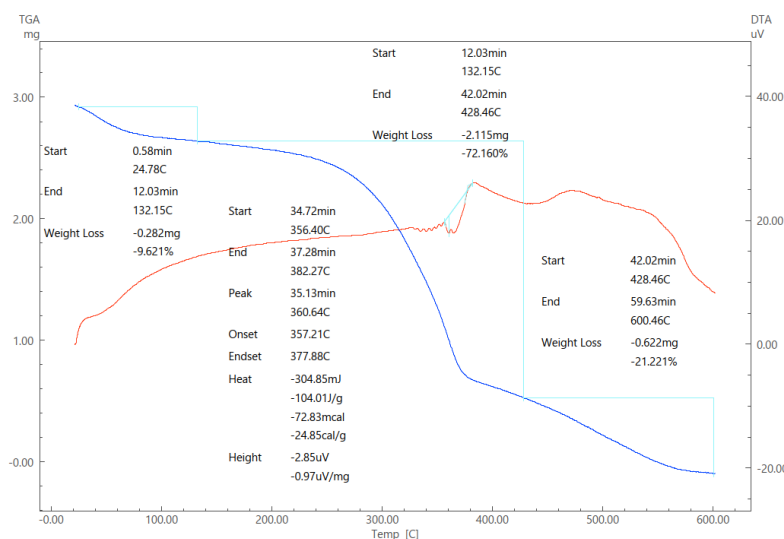
Figure 2. Thermal stability of wood materials treated with PO-2 brand flame retardant
