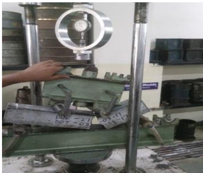
Fig. 5- after testing of prism sample for flexural strength
