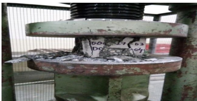
fig. 1 specimen subjected to Compressive strength for high strength Traditionally vibrated concrete (M60)
