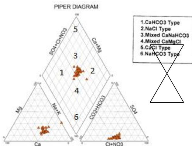
**Figure 4. Piper diagram for hydrochemical facies**
