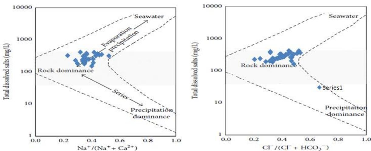
**Figure 6. Gibbs diagram showing the process affecting groundwater chemistry**
