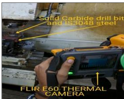
Fig. 1 Experimental Setup in Drilling of IS3048 Steel
