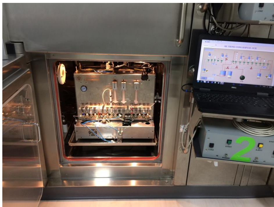
Figure 1. Home-made full automatic synthesizer for ^{18}\text{F} FCH production
