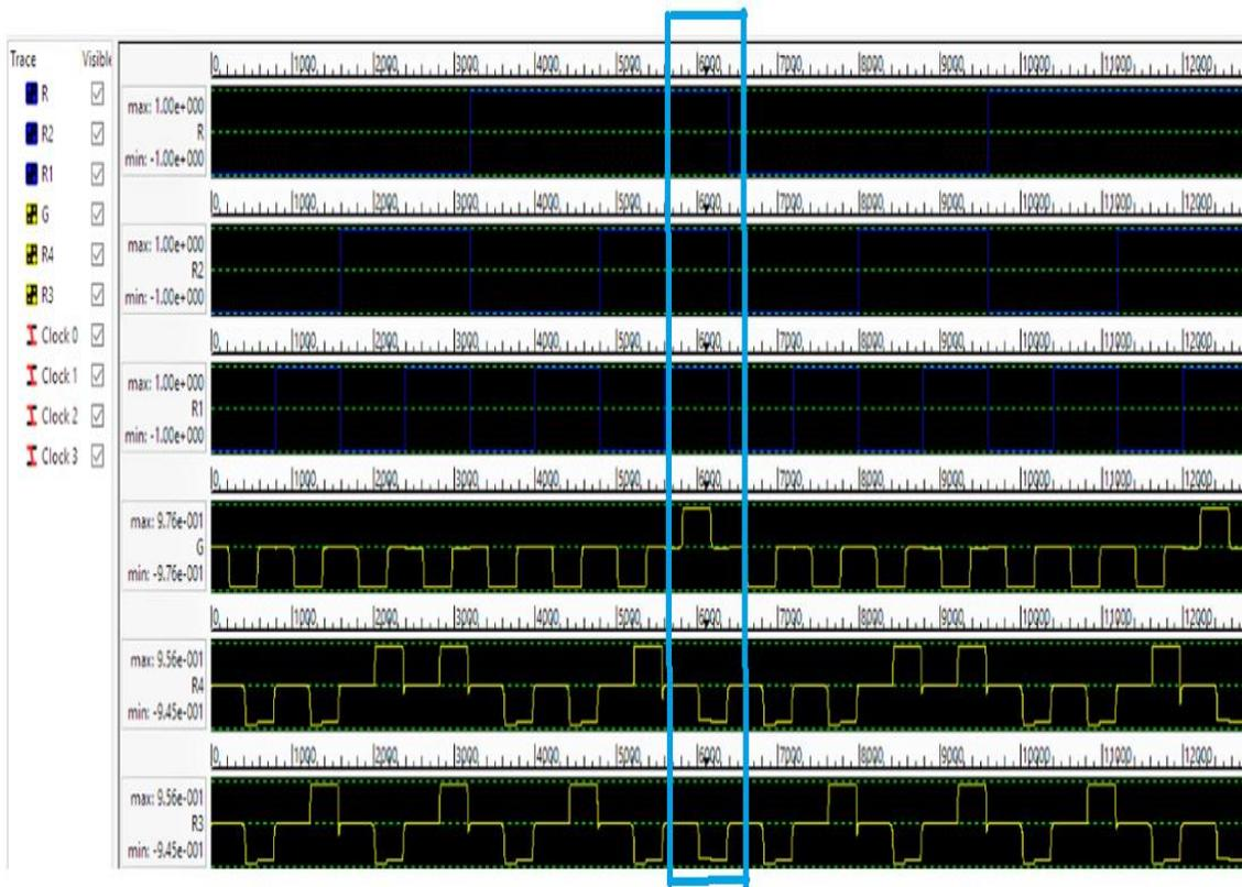
Figure 12 The simulation result of cell scheduler under 2-DW clocking scheme
