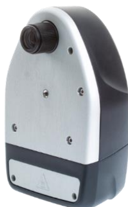
Figure 2: Photo of Senop HSC-2 Hyperspectral Camera
