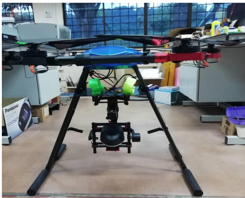
Figure 8: Payload tray mounted with batteries and gimbal
