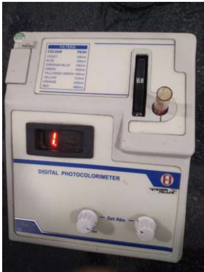
Fig 2: The figure shows digital photo colorimeter to measure the absorbance of extract at 517 nm of wavelength
