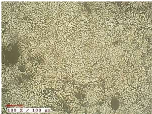
Figure 2 91% of Al and 5% of B 4 C,4% of Graphite Graphite
