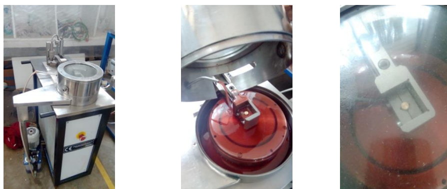
Fig 2: Experimental setup for lubricated sliding wear studies
