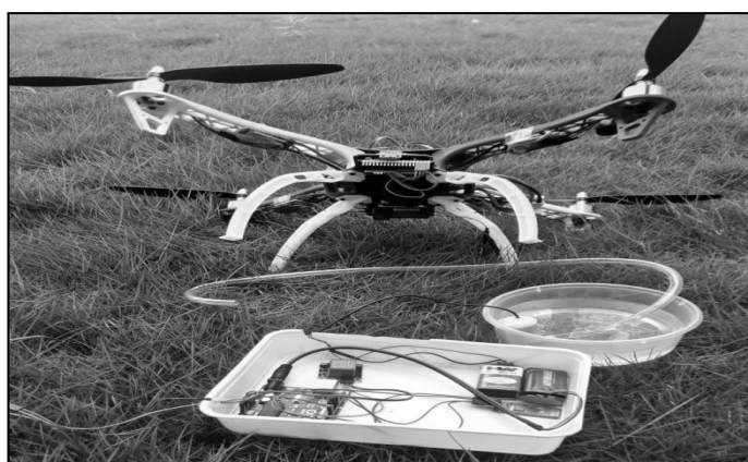
Figure.16. Prototype module of agriculture machinery control and monitoring system with IoT
