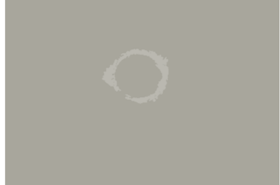
Figure 5. Threshold Image of a Drilled Hole
