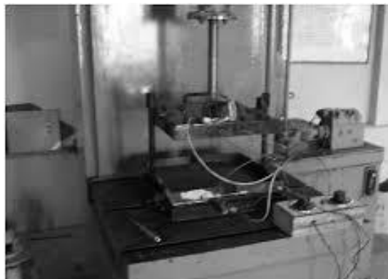
Figure 2. Drilling of Composite in Vertical Milling Machine
