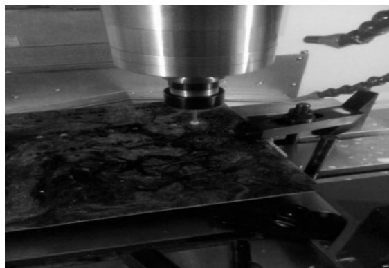
Figure 2. Drilling of Composite in Vertical Milling Machine
