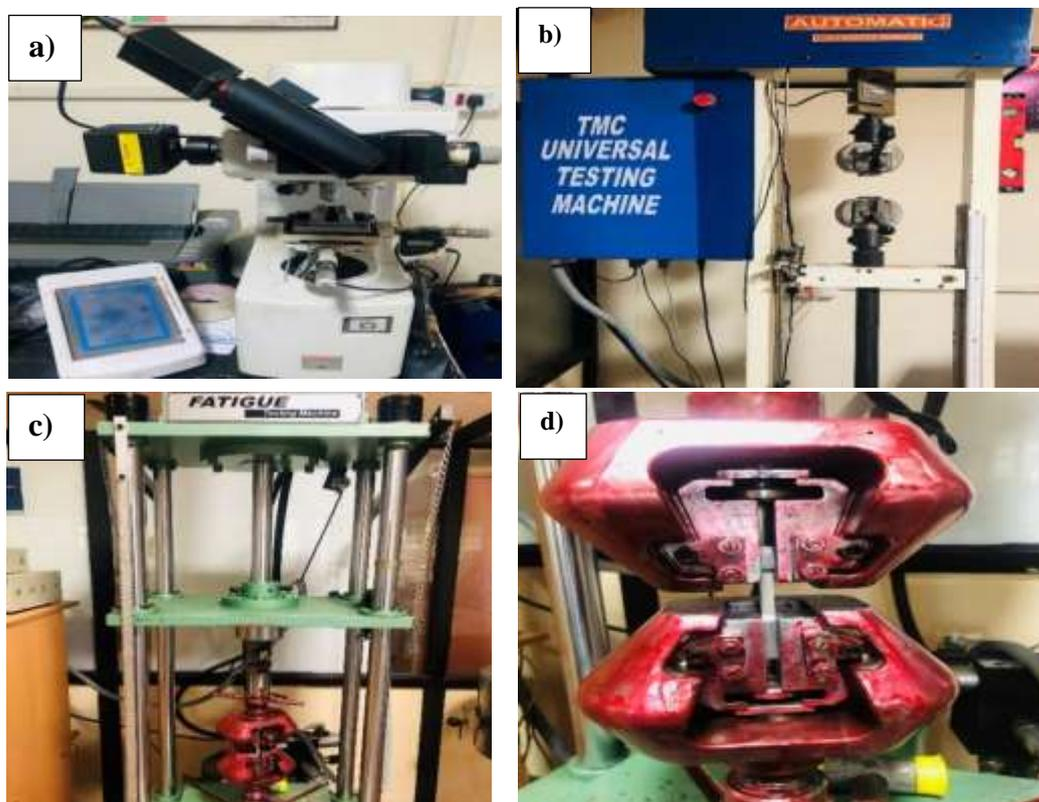
Fig 1. a) Micro Hardness Tester b) Universal Testing Machine c) Fatigue Testing Machine d) Fatigue test specimen holder
