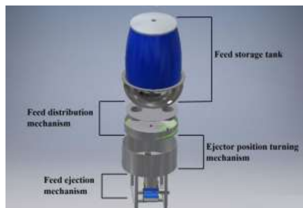
Fig.3. Feed storage tank and the three mechanisms of the fish feeding robot prototype
