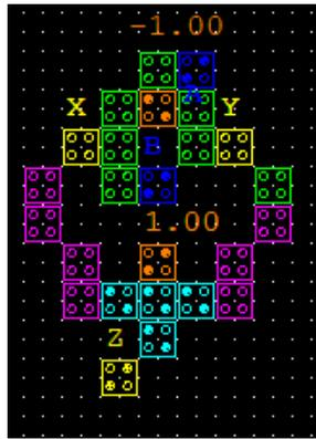
The simulations are done using QCA Designer tool. As illustrated in the figure 7 when the inputs A and B equals to logic 01 then  $A < B$  which can be shown by the output X, when the inputs A and B equals to logic 10 then  $A > B$  which is shown by output Y and inputs A and B equals to logic 00 or logic 11 then the inputs  $A = B$  which is shown by output Z.
