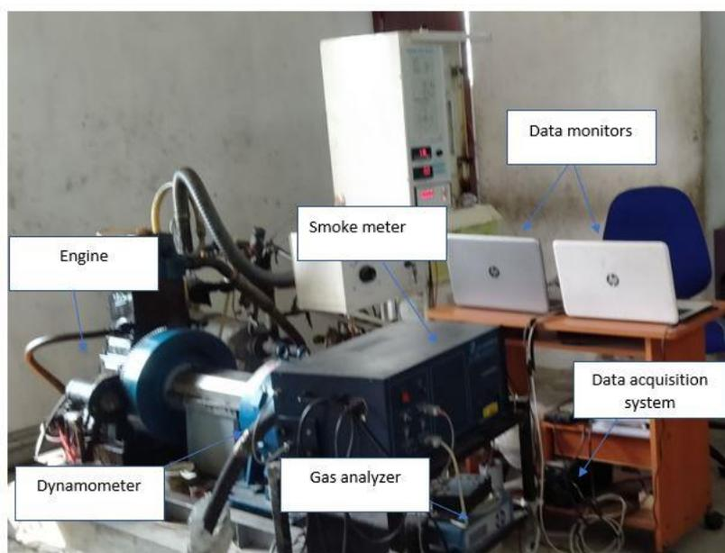
Fig 2. Photograph of CI Engine
