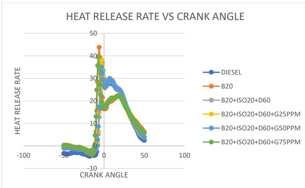
Fig 6. Heat release rate vs crank angle at full load
