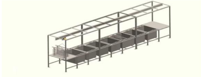
Figure 11. Pre-Treatment Process System Model
