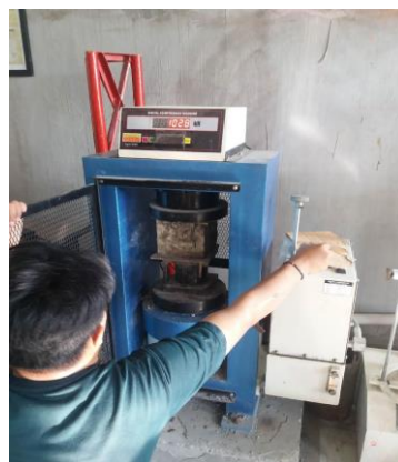
(b) Compressive test set-up
