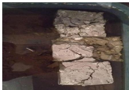
The specimens at surface & around the edges were lightly broken. Some fine cracks and aggregates were distinctly noticeable. The specimens after 30 days of exposure to solution of 5% sulphuric acid was not that much distorted though collated to 60 and 90 days of immersion. Geopolymer Concrete cube specimens had loss in its strength after 30, 60 and 90 days after exposure to H<sub>2</sub>SO<sub>4</sub> solution. This possibly ascribed to
