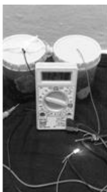
Fig 11: Glowing led by Voltage Generation
