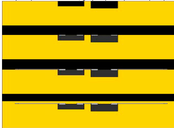
Figure 4: From top to bottom: printing object with cavities and channels, placing components, making conductive tracks, continue printing of the object. (Source :[18])
