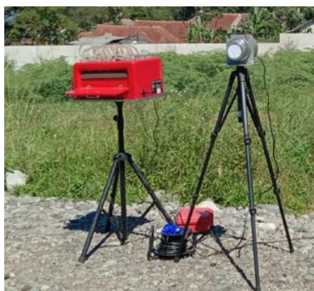
Fig. 1. Gravimetric, gas analyzer, and sound level meter device
