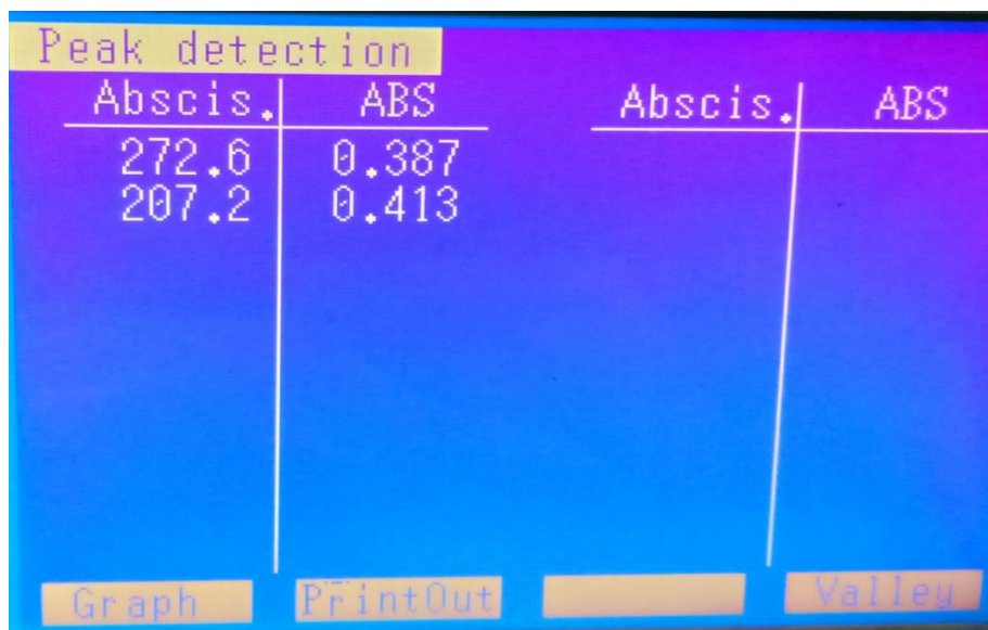
Figure 2- U.V. Spectroscopy of the Doxycycline
