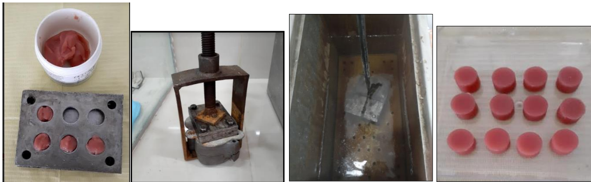
Picture 2. Making of heat-cured silicone soft denture liner samples
