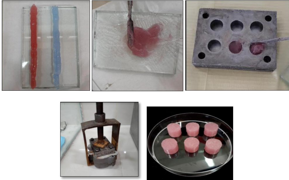
Picture 1. Making of self-cured silicone soft denture liner samples
