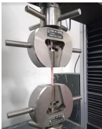
Figure 5 Tensile Strength Testing with UTM Tensilometer, AND, RTF – 1350, Japan
