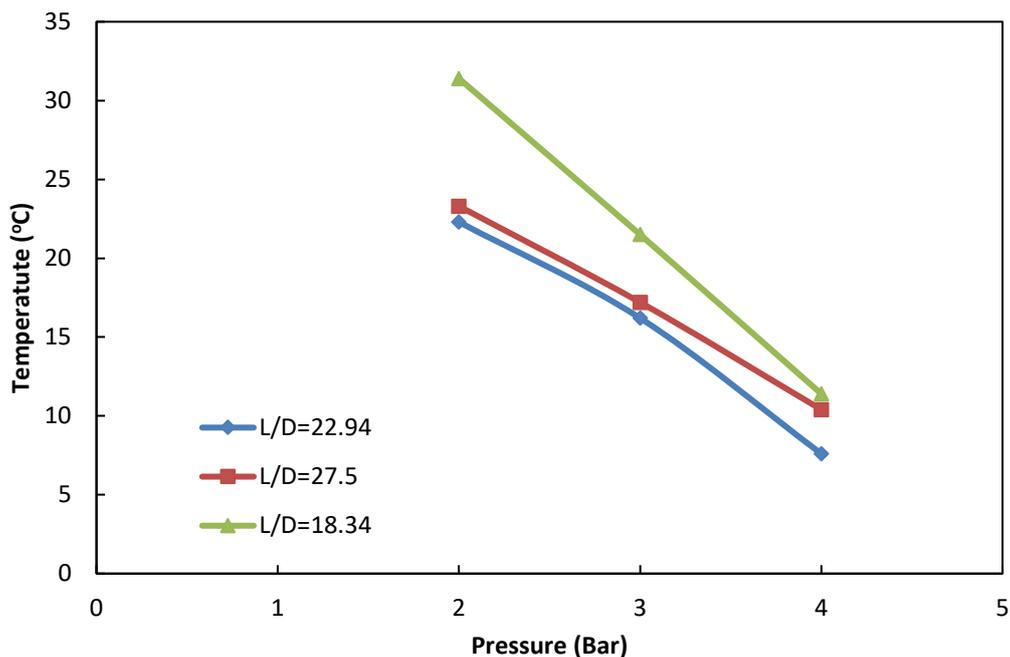
**Figure 3. Variation of cold stream temperature with air pressure**
