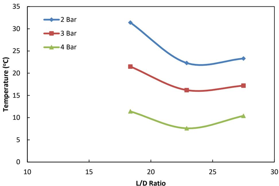
**Figure 4. Variation of cold stream temperature with L/D ratio**
