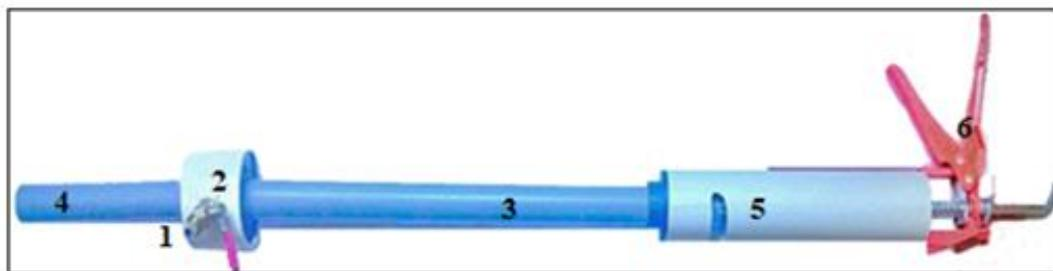
**Figure 2. The locally fabricated vortex tube**
