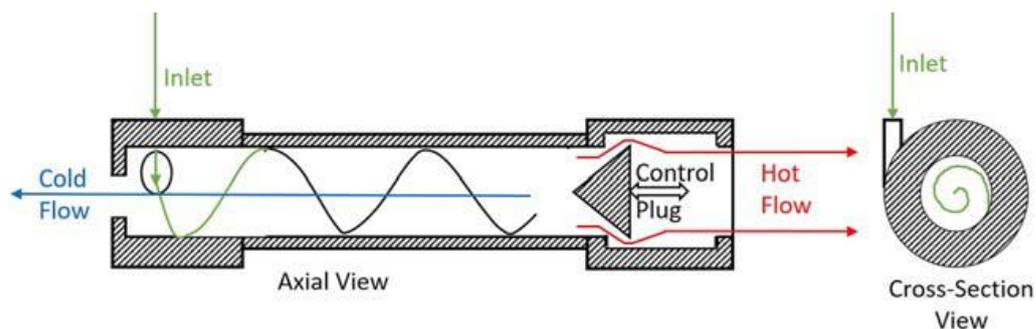
**Figure 1. Flow structure in a counter-flow vortex tube [10]**
