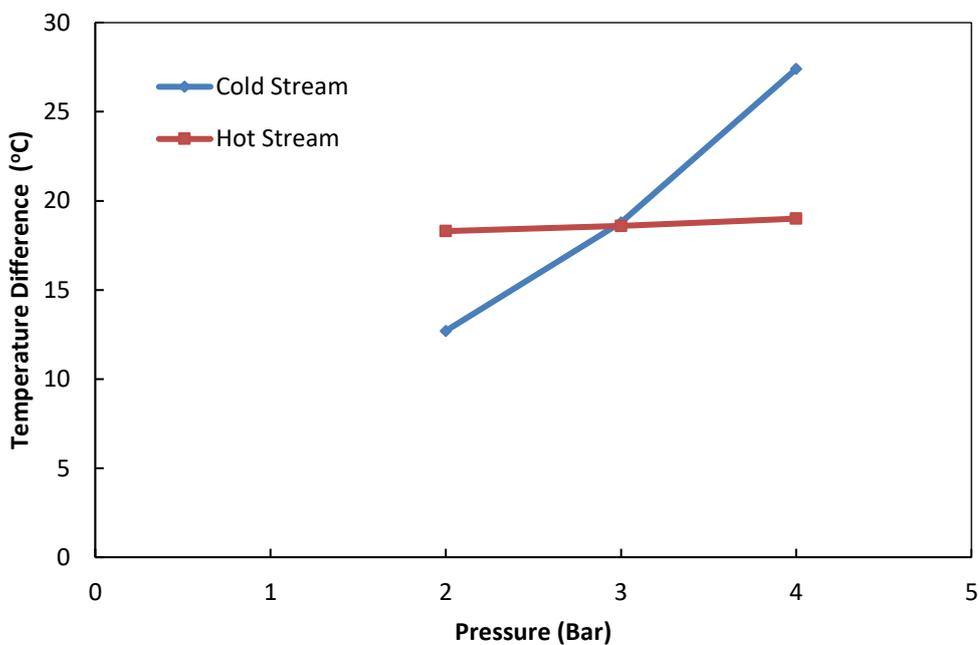
**Figure 6. Comparison on temperature difference for hot and cold streams at L/D ratio of 22.94**
