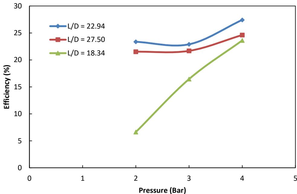
**Figure 7. Variation of isentropic efficiency with pressure for L/D ratio**
