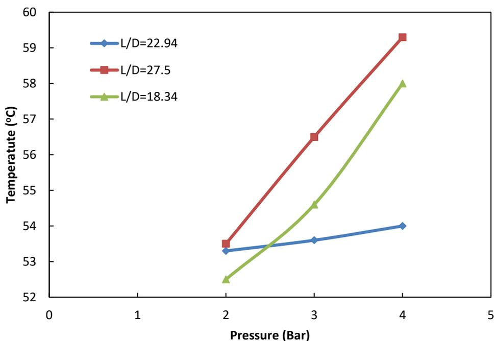
**Figure 5. Variation of hot stream temperature with air pressure**
