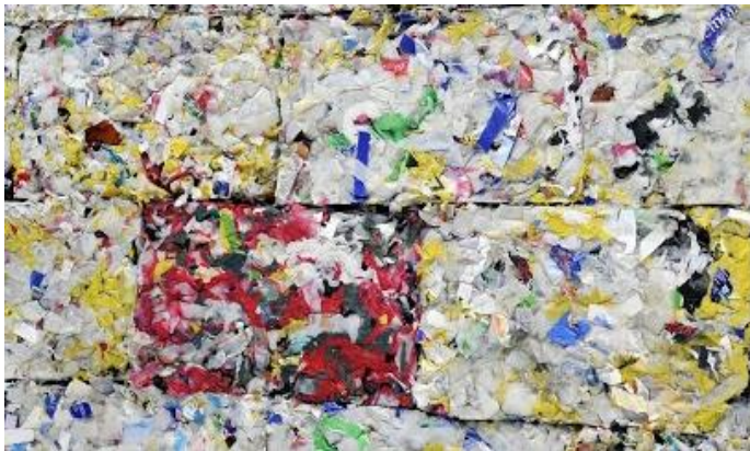
Fig 11: Building blocks using plastic waste
