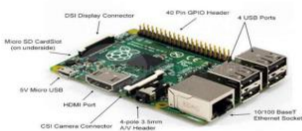
Figure 2.1: Raspberry pi embedded board.
