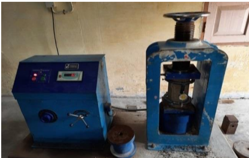
Figure 4: Test setup for Modulus of elasticity
