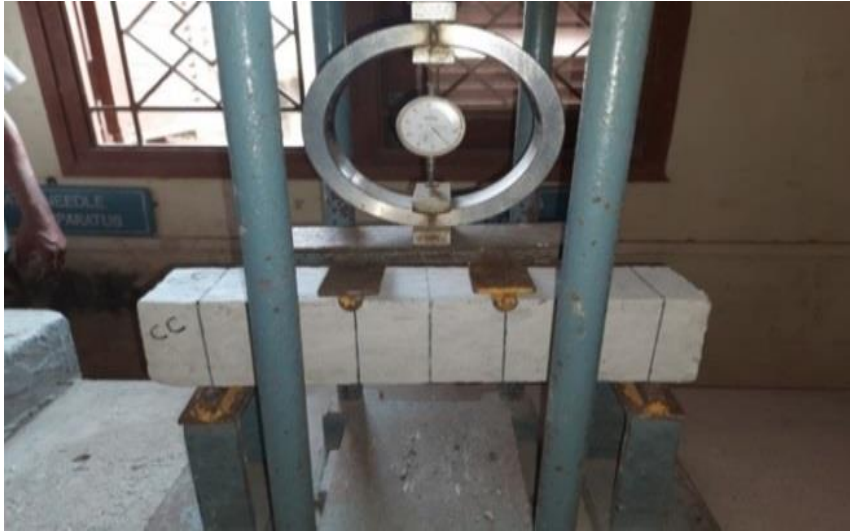
Figure 3: Test setup for Flexural strength
