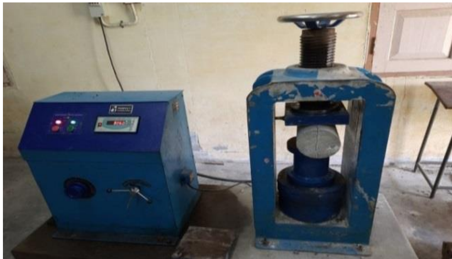
Figure 2: Test setup for Split tensile strength
