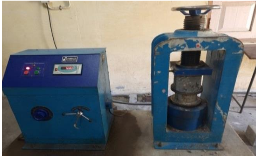
Figure 1: Test setup for Compressive strength
