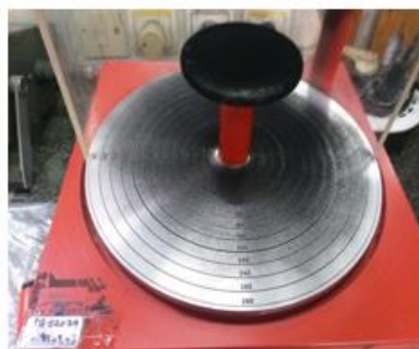
Fig 2: Nano-composite flock sample spraying test, Fig 3: Flock sample spraying test alone
