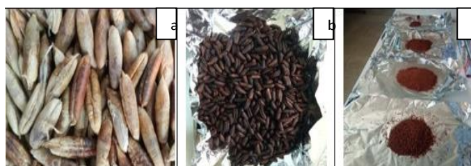
Figure 2. Photographs of organic matrix preparation The raw material (a) After the carbonization process (b) organic matrix (c)
