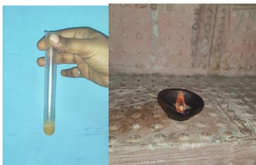
Figure 9: Microbial seed oil and Sand pot used for flame testing
