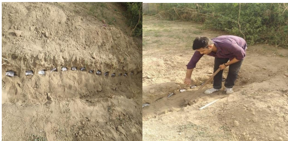
Fig. 1 and 2 Placement of Samples at experimental site
