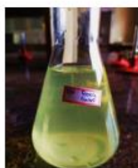
Colour transformation of the 1mM Cu (NO 3 ) 2 solution with the addition of P. fruticosus root saponin extract
