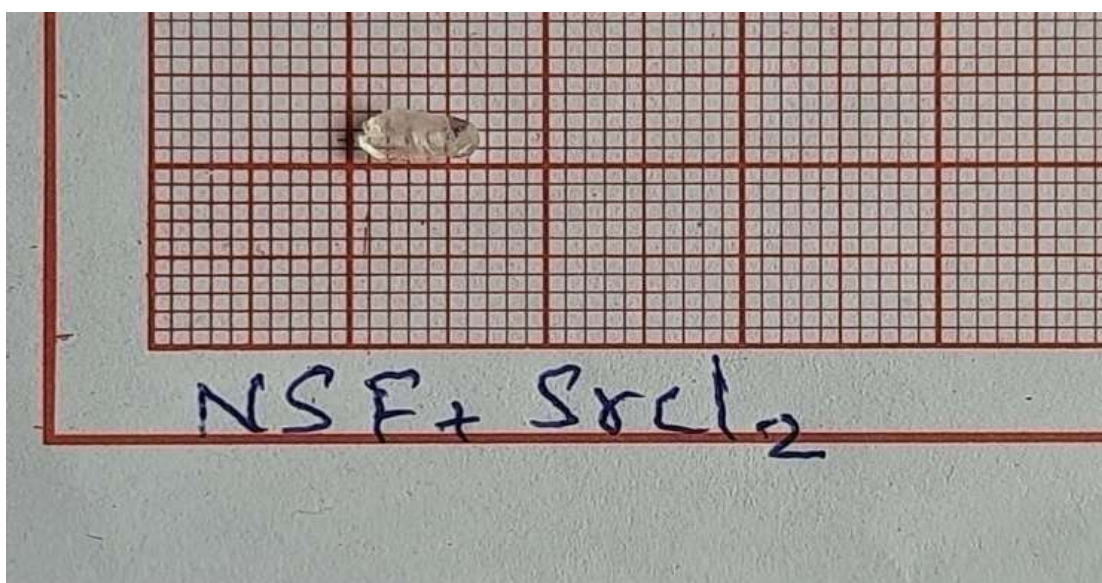
Fig.1 Photograph of grown (Na) 2 SbF 5 single crystal
