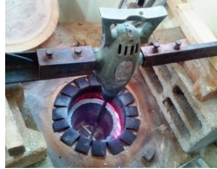
Fig.2 Custom made in-house stirrer
