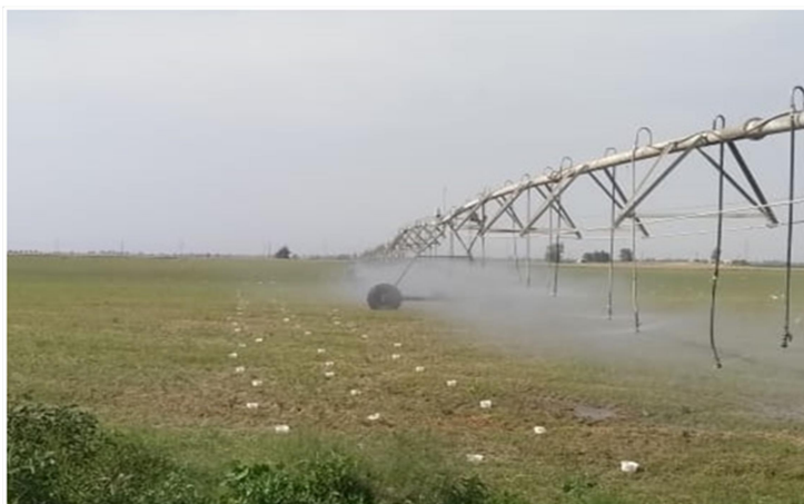
Fig. 2. Center pivot and catch cans distribution lines.
