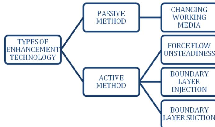
**Figure 1 Types of Methods used for Heat Transfer Enhancement in a Microchannel.**
