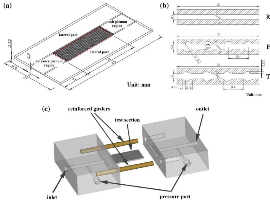
**Figure 2 (a) Structure of heat sink (b) size of heat sink (c) packaging of the system.[10].**
