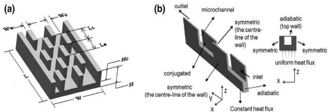
**Figure 4 Schematic Diagram of (a) Offset Strip-fin (b) Computational Domain [13].**
