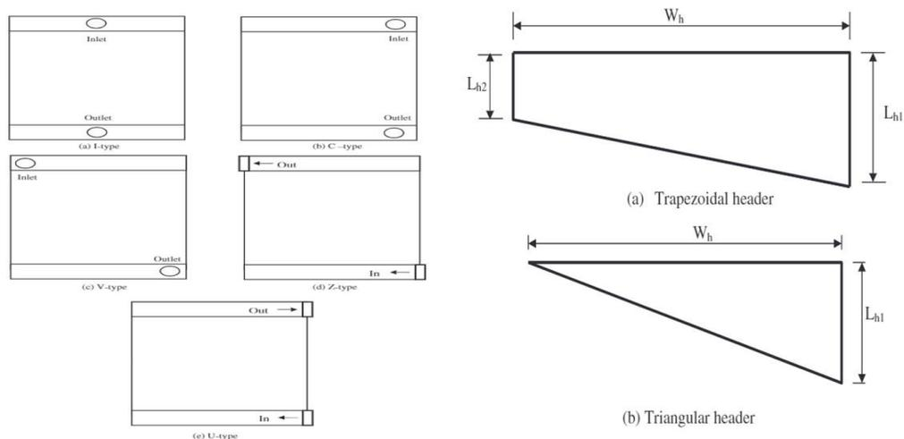
**Figure 7** Schematic diagram of micro-channel with (1) Different inlet-outlet configurations (2) different header shapes [28].
