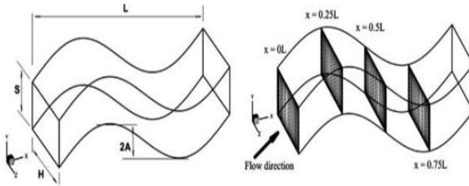
**Figure 5** Geometry of Three-Dimensional Sinusoidal wavy-Plate-fin. [15].
