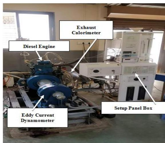
The investigations were carried out at the dedicated Research Associated Lab (RAL) at Apex Innovations Pvt. Ltd. Sangali, Maharashtra, India. . The crank driven supercharger, turbocharger and electric supercharger combined assembly is shown in Fig.2. The setup consists of a single-cylinder, four-stroke, diesel engine connected to an eddy current dynamometer, computerised model-224 shown in
