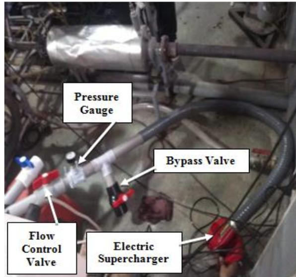
Figure 7. Tri-charged Engine Setup
