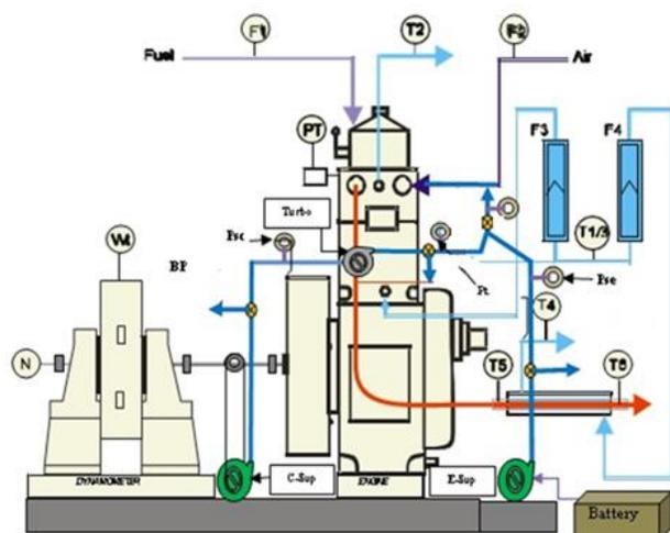
**Figure 3. Single Cylinder 4-Stroke VCR (Computerised) Test Rig**
