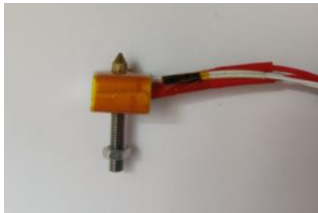
Fig 6 Hot end of extruder
