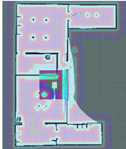
Fig 16. Google cartographer mapping
