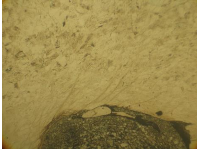
Fig. 20 Clad interface changes for a given heat input
