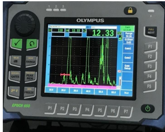
Fig. 3 Instance of artificial debonding
