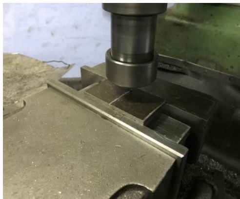
Fig. 7 Grooves machined using end mill cutter
