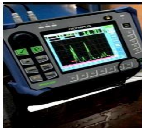
Fig. 4 Instance of backwall loss due to subsurface defect
