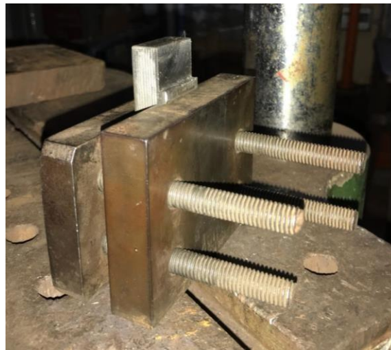
Fig. 14 Setup for Shear testing
