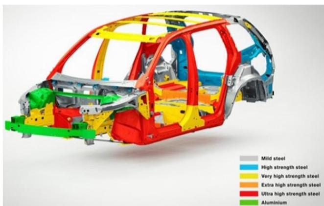
Figure 3. Materials utilised in the new Volvo XC90 (Courtesy of Volvo Car Corporation)
