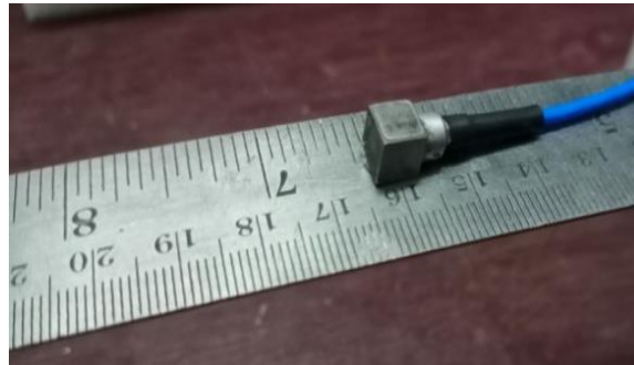
Figure 3. Accelerometer used in detecting damping vibrations in a ruler
