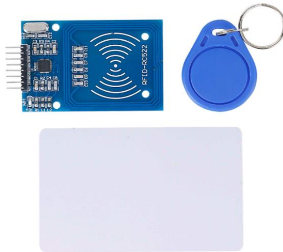
Fig. 2. RFID reader module with white card and key ring
