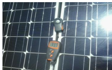
Fig 14 Irradiation measurement using flux meter
