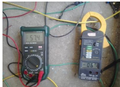
Fig 13 voltage and Current Measurement
