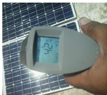
Fig 14 Irradiation measurement using flux meter
