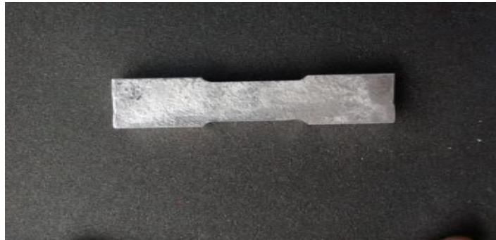
Fig. 12 Fabricated tensile test specimen.
